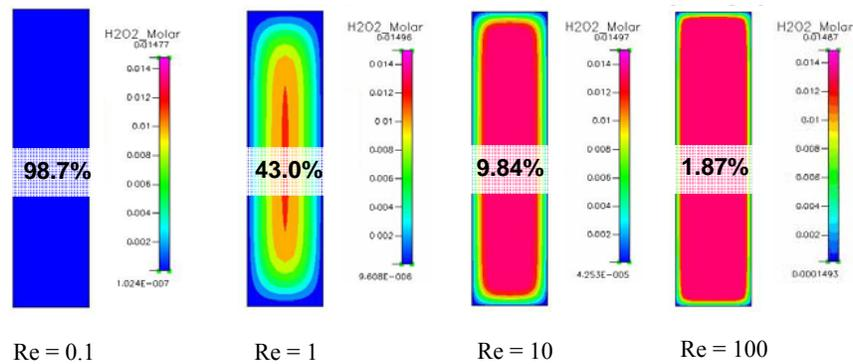
**Figure 3. Outlet Conversion Fields of the Empty Channel at Various Reynolds Numbers**
