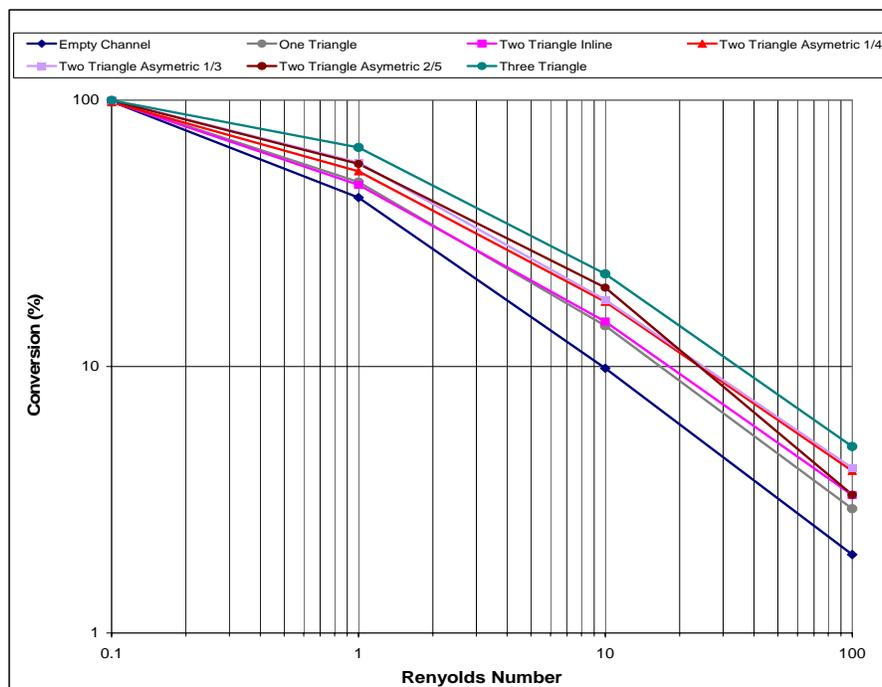
**Figure 5. Log-Log Plot of Conversion versus Reynolds Number for Each Configuration**
