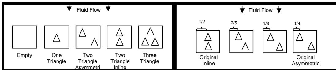
**Figure 2. Microchannel Obstruction Configurations**
