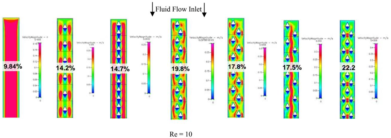
**Figure 4. Top View of the Various Packed Channels Showing Velocity Fields at Re = 10**
