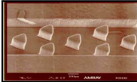
**Figure 1. SEM of PDMS Microchannel Used in Physical Experimentation [2]**
